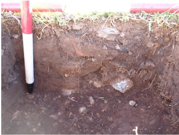
Figure 79 – Section of TP C1 showing high level of disturbance with concrete, rock and gravel inclusions.
